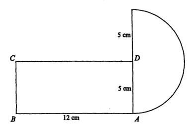
(ii) Calculate the distance of the centre of mass of the combined object from the point B.
