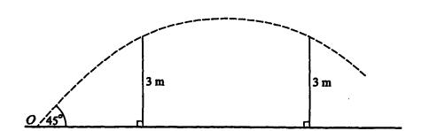
Two thin poles of height 3 m stand vertically in the plane of the path of the particle. When  $\theta = 45^{\circ}$ , the particle just passes over the tops of both poles (see diagram).
